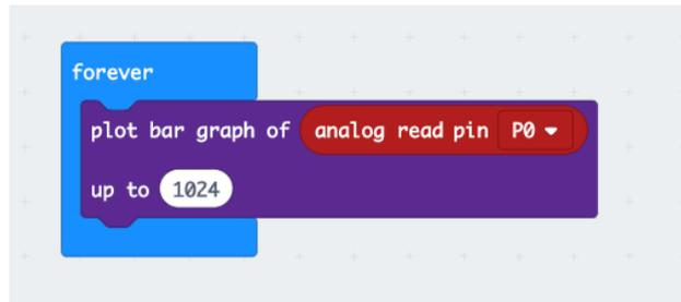
This code will show a bar graph of the input the micro:bit receives from the input part on port 0. Trigger the sensor to see how the micro:bit responds.
